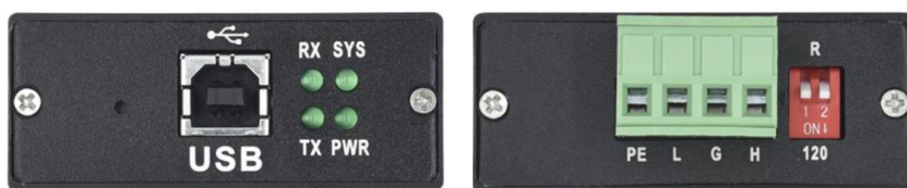
(a) USB Port (b) CAN-bus Port Figure 2-2 “eRob to PC Connector” Port Illustration
